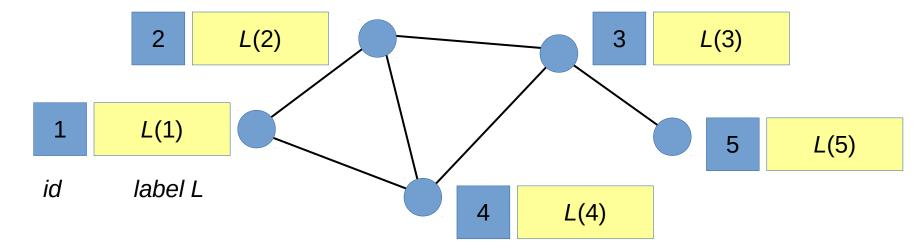
**The decoder** must be able to process a distance query based only on the labels of the involved nodes.
